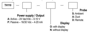
**Example: TH110 – ANS** Humidity and temperature transmitter TH110, 0-10 V active, without display, ambient model
