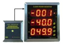
**Accuracy**  $\pm 0.5^{\circ}\text{C}$  for Temperature,
