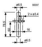
2 duct adaptors and 2 m tubing are supplied with the pressure switch.
