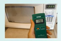
Easy-to-use, compact microwave leakage detector designed to measure high frequency radiation levels emitted from household and commercial microwave ovens.
