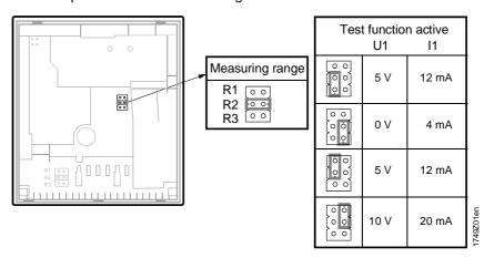
The setting element is accessible after removing the baseplate.
