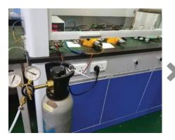
Factory Calibration The sensors are bump tested at Oizom factory to check their proper functioning for each parameter.
