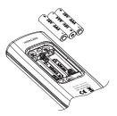
Replace the battery cover making sure that the gasket is in place.
