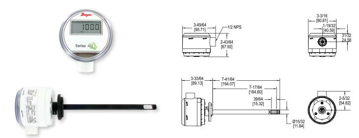
The **SERIES AVUL** Air Velocity Transmitter quickly and accurately measures air velocity or volumetric flow in imperial or metric units. Simultaneous current and voltage outputs on all models provide universal inputs to monitoring equipment while the output range, units, and 0 to 5/10 VDC output can be configured via local DIP switches. The optional integral display, or the portable remote display tool, provide a convenient way to locally monitor process values and configure the unit.
