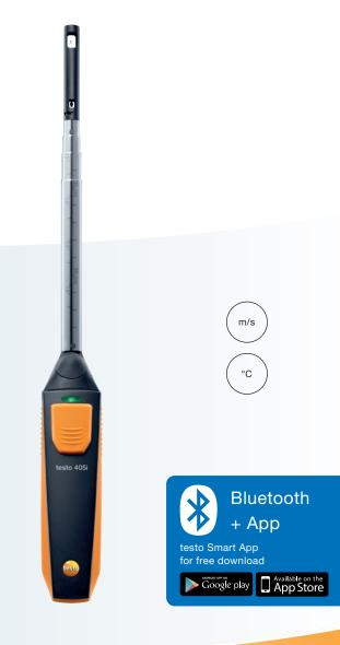
The hot-wire anemometer testo 405i, in combination with a smartphone or tablet, is a compact measuring instrument for air flow velocities, temperatures and volume flows. Equipped with a telescopic shaft, extendable to 400 mm, it allows flexible applications in rooms and ducts. Via the testo Smart App installed on the end device, users can comfortably read off their measurement values, configure volume flow measurements quickly and easily, and reliably determine timed and multi-point mean values.
