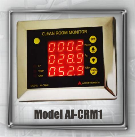
The **Clean Room Monitor** is designed to measure the vital parameters of Temperature, Humidity & Differential Pressure in Clean Room application.
