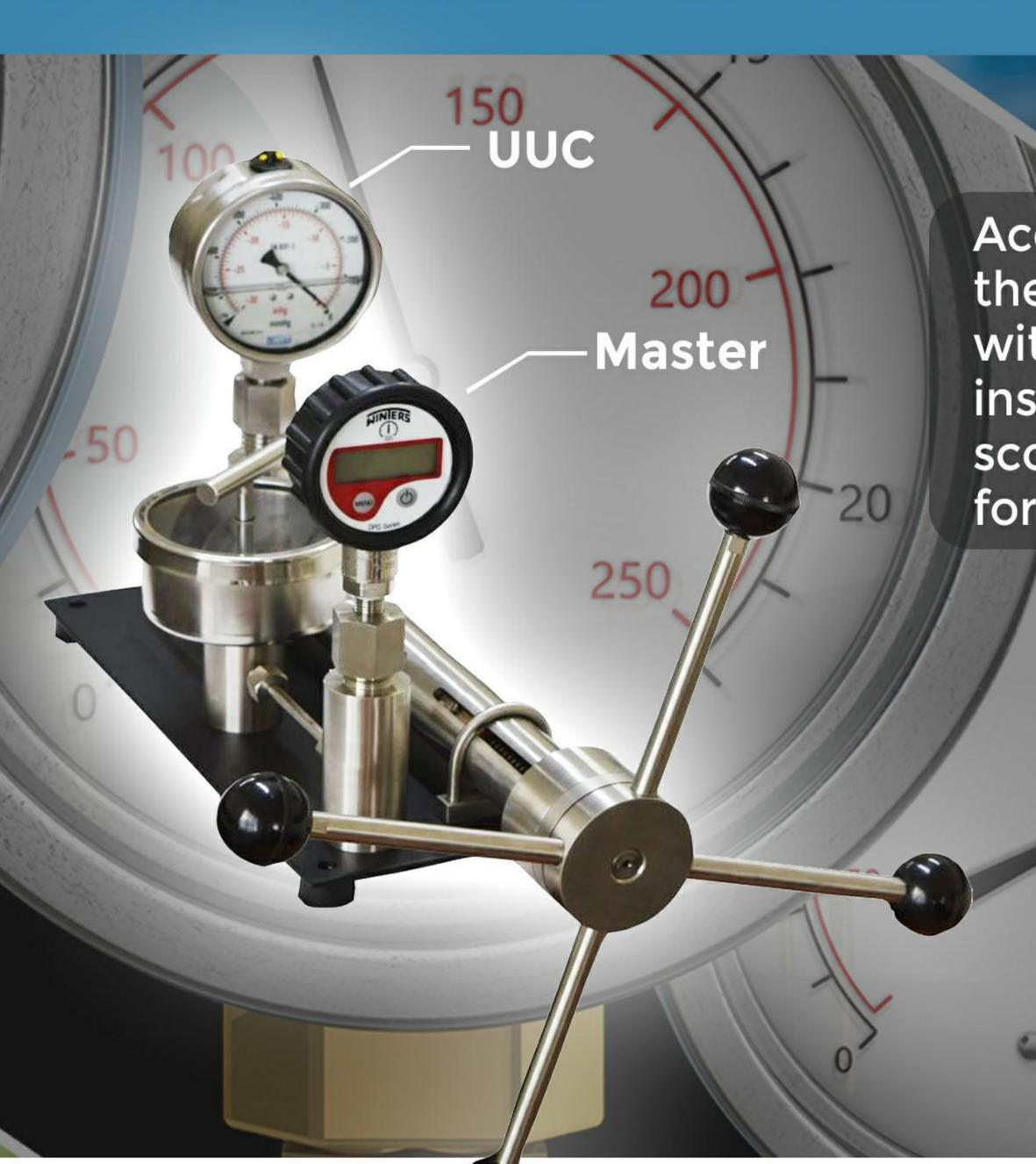
Ace AI-PCAL1 Pressure & Vaccum Calibrator is used to generate the required pressure for calibrating the pressure instruments with a comparison method. In this method generally, pressure instruments are calibrated against a master instrument. The scope of reference calibration is to minimize the time required for calibrating a pressure instrument.
