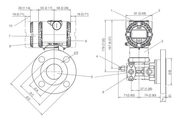
NOTE: Process connection, gasket groove and gaskets are in accordance with IEC 61518. Bolting threads for fixing adapter or other devices (i.e. manifold etc.) on process flange is  $^{7}/_{16}$  – 20 UNF.
